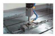
Crystal Brite was developed to improve the spark erosion process in sinker style EDM machines. It has allowed users to increase amperage, thus reducing process times by as much as 30%. Also, it creates a non-conductive channel allowing the spark to hit its target accurately and at a full charge. It reduces carbonization, which reduces gummy residue.
